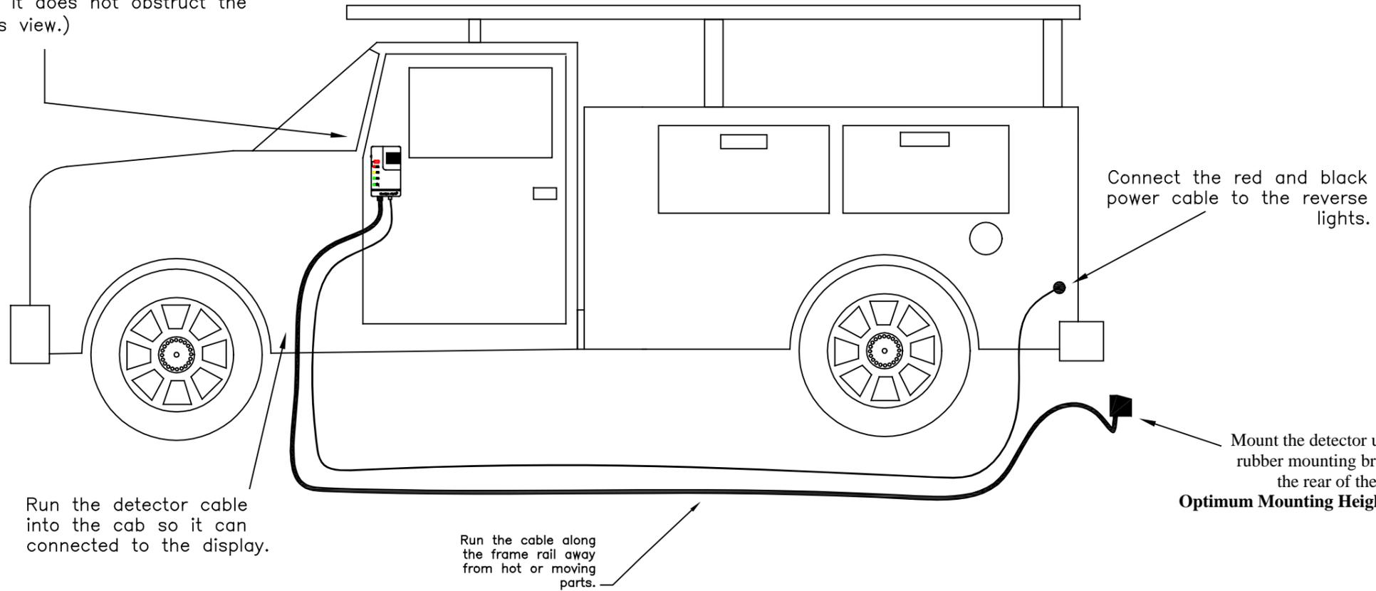
Mount the detector using the rubber mounting bracket on the rear of the vehicle.
